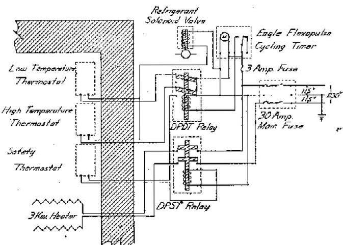
Fig. 1 Control system for automatically fluctuating the temperature of a refrigerator
