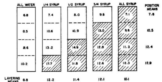
Figure 2. Average heating rates,  $f_h$ , min, in water-syrup (50% sucrose) model systems.
