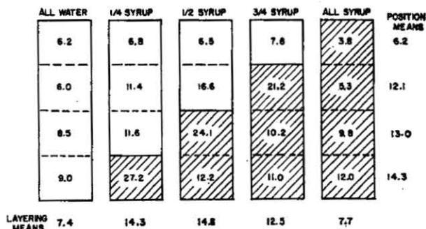
Figure 4. Average heating rates,  $f_h$  min, in water-syrup (50% sucrose) model systems with plastic spears.
