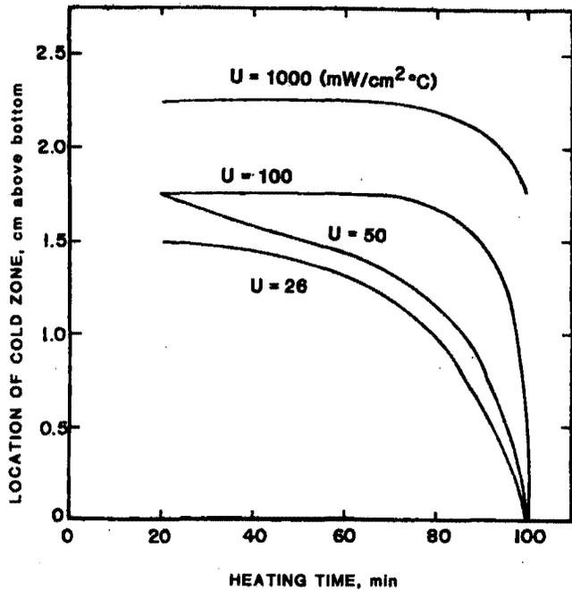
Fig. 5—Location of the moving cold zone (height above can bottom) for a conduction heating product ( $\alpha = 0.0016 \text{ cm}^2/\text{sec}$ ) in a 401 x 204 can as a function of heating time and the heat transfer coefficient between steam and bottom plate. Results of computer simulations.
