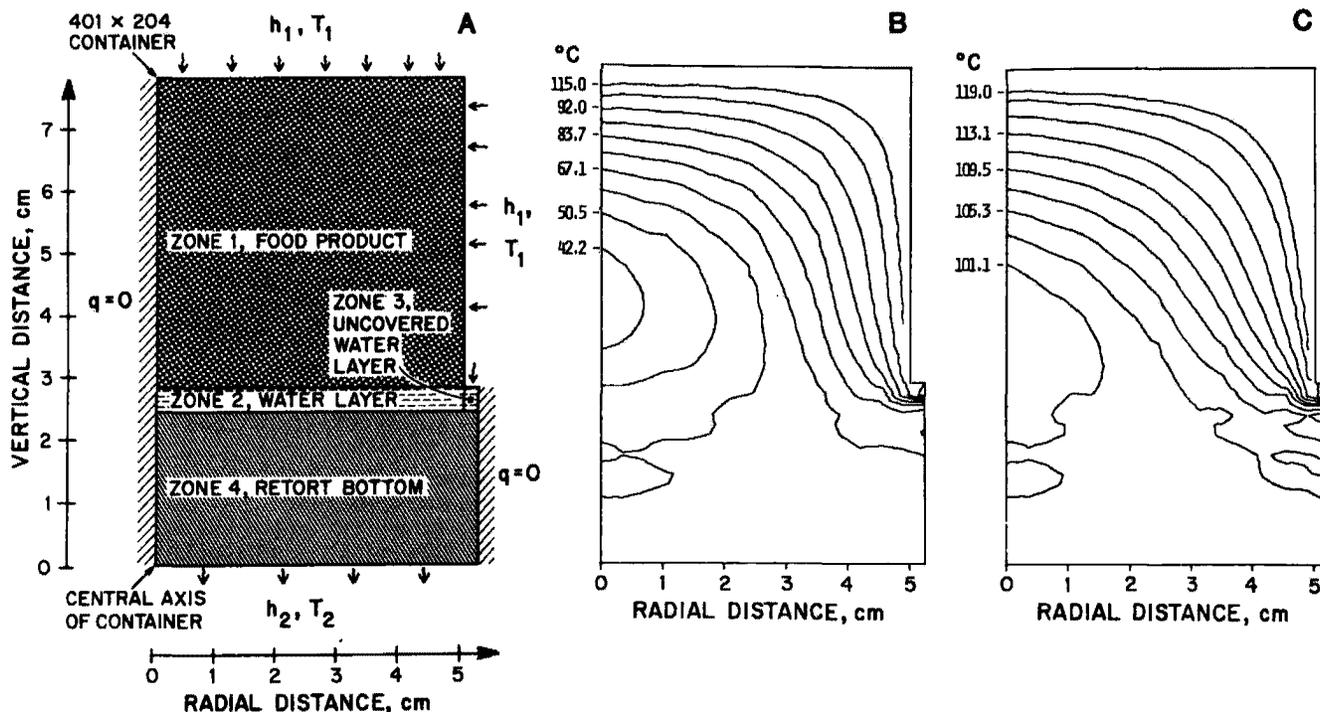
Fig. 1—Container with one end flat against retort bottom: (A) Zones and boundary conditions; (B) Isotherms obtained from numerical solution after heating time of 20.3 min; (C) After 70.3 min.
