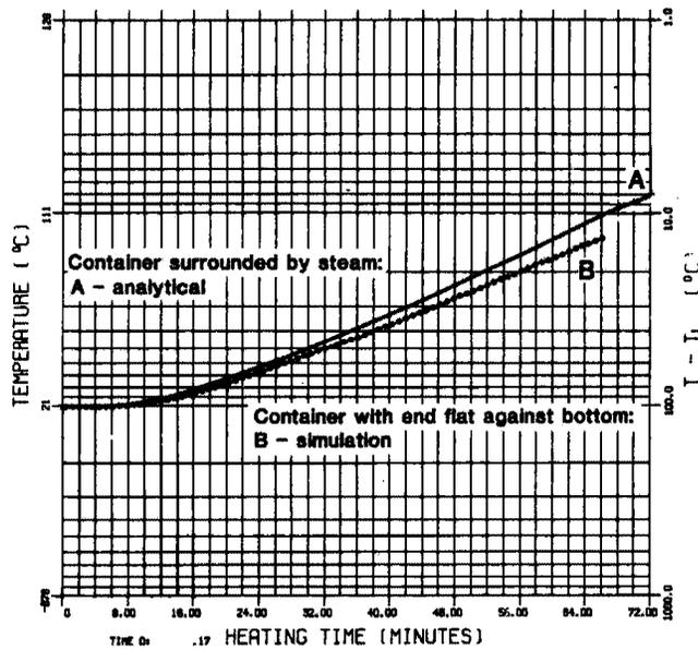
Fig. 3—Heating curves (geometric center) for 303 x 406 can filled with a water-like conduction heating product ( $\alpha = 0.0016 \text{ cm}^2/\text{sec}$ ).
