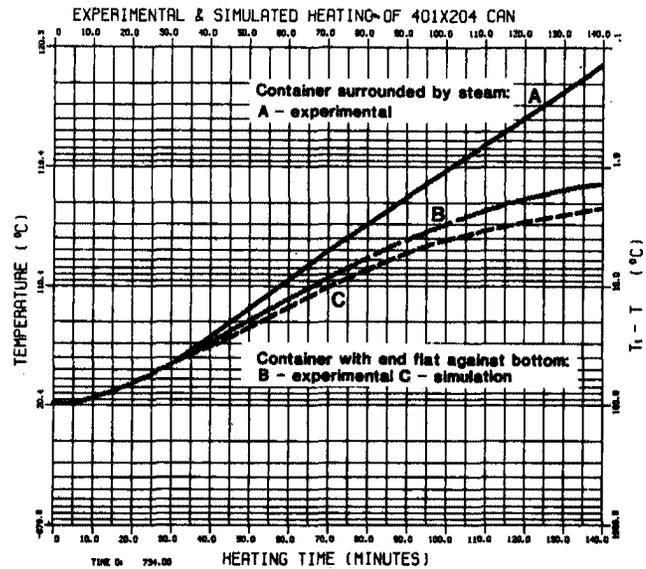
Fig. 6—Heating curves obtained in laboratory test chamber, A and B; and C, Results of computer simulations assuming a heat transfer coefficient of 50  $\text{mW}/\text{cm}^2\text{C}$  between retort bottom and steam.
