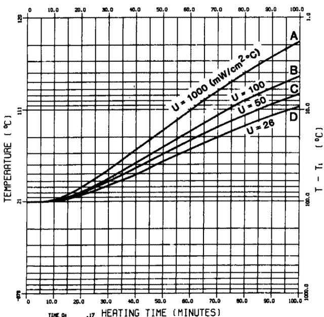
Fig. 4—Heating curves (geometric center) for 401 x 204 can with end flat against retort bottom for different values of heat transfer coefficients between steam and bottom plate.
