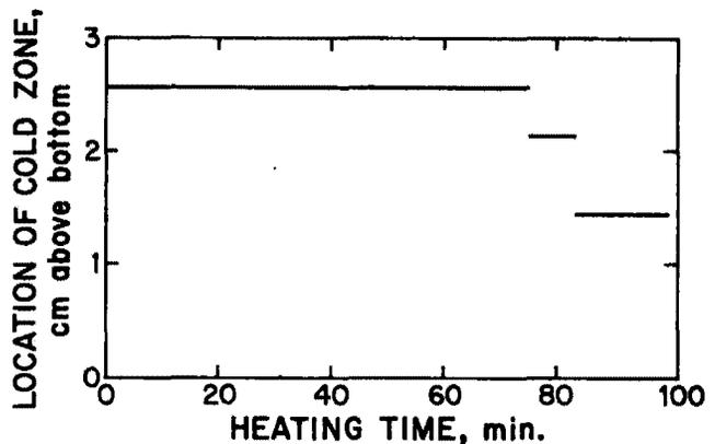
Fig. 7—Location of the lowest reading thermocouple in a 401 x 204 can filled with a starch paste heated with an end flat against the bottom of the laboratory steam chamber.
