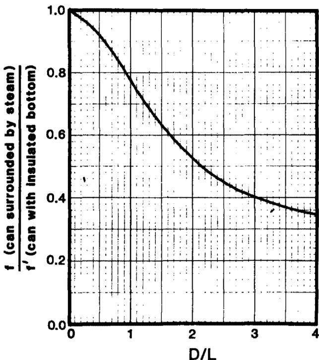
Fig. 2—Ratio of  $f$  of can surrounded by steam to  $f$  of can with insulated bottom as a function of the container length to diameter ratio. Results based on analytical solution.
